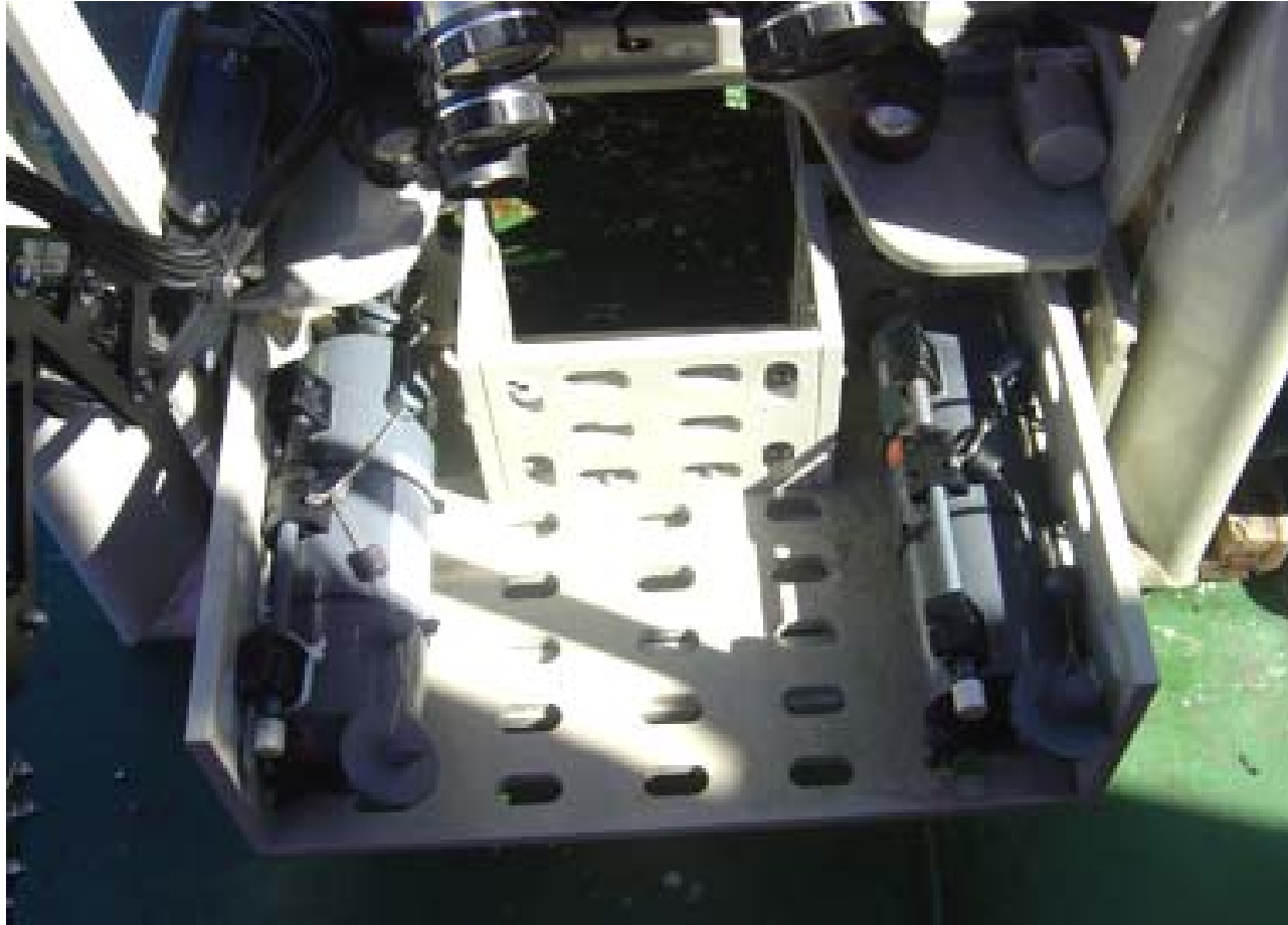
2 Niskin water-sample bottles mounted in the sample tray. They can be closed by the operator at any time and location by the manipulator arm.
