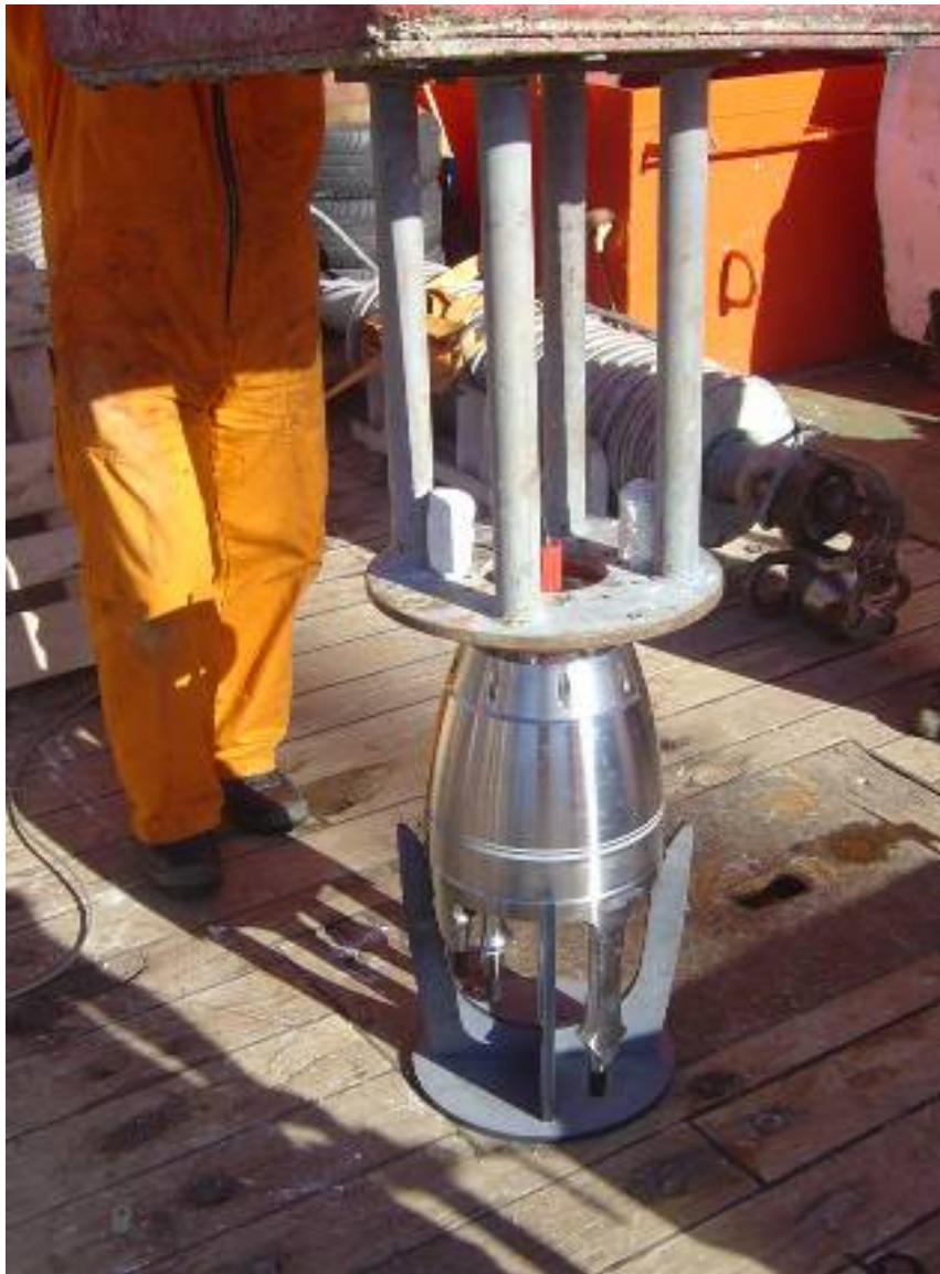
Meter-scale positioning and navigation with ship-mounted IXSEA GAPS (picture above) and 2 ROV-mounted and TMS-mounted transponders
