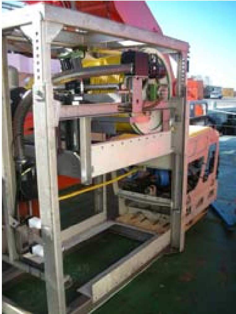
The ROV + TMS on deck. On these pictures, the ROV has been moved out of the TMS slot for maintenance and control purposes.
