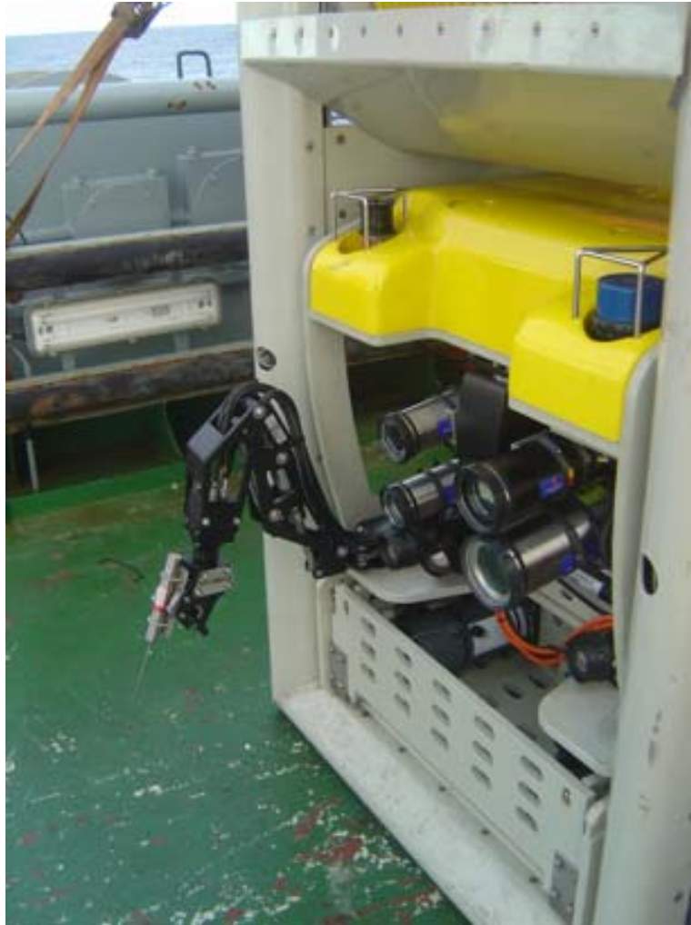
THP thermistor mounted on the manipulator arm to conduct sea-floor temperature measurements at seep locations
