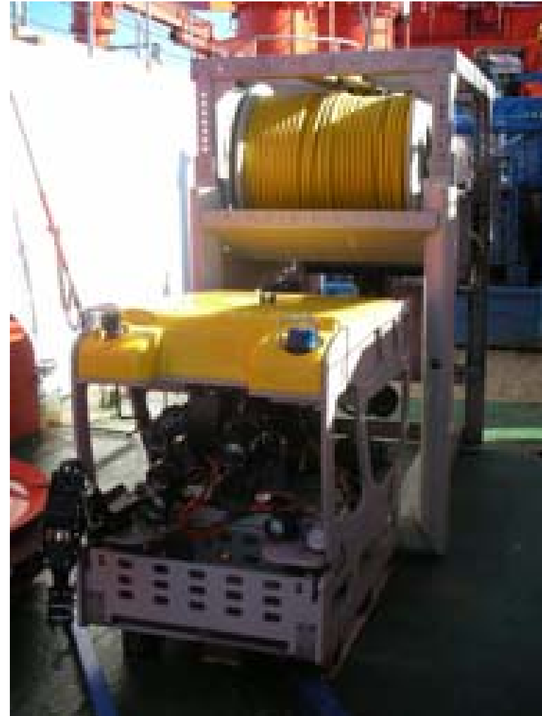
The ROV + TMS on deck. On these pictures, the ROV has been moved out of the TMS slot for maintenance and control purposes.
