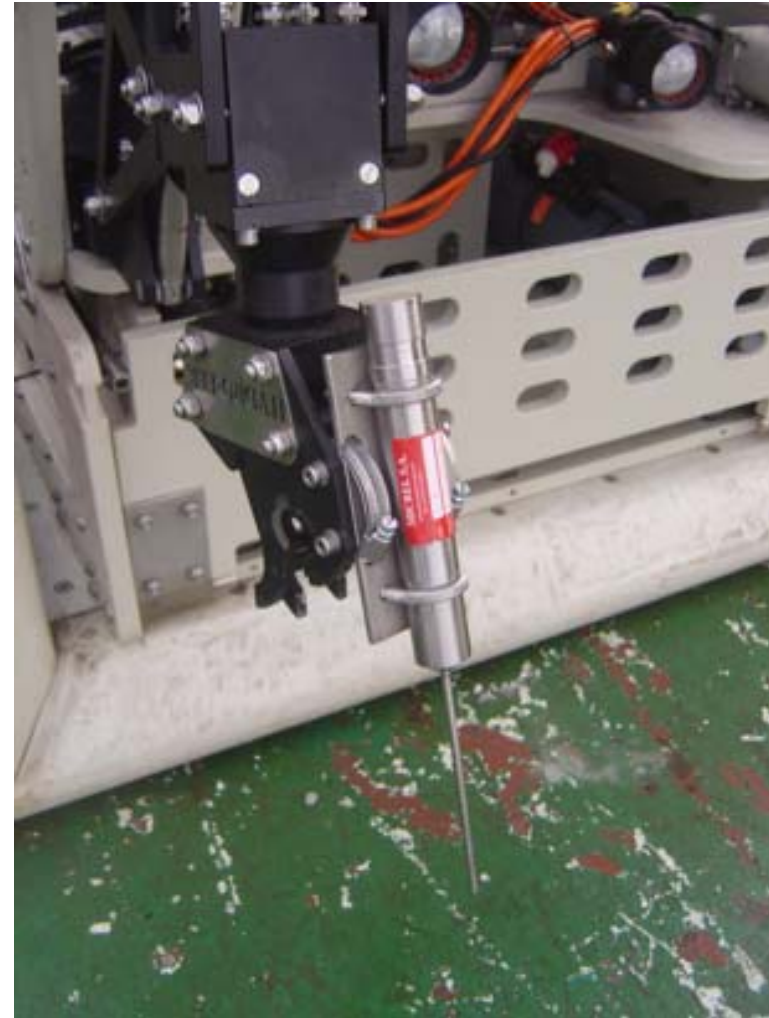
THP thermistor mounted on the manipulator arm to conduct sea-floor temperature measurements at seep locations
